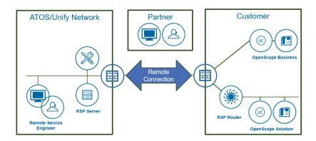
RSP provides a connectivity type called RSP.servicelink (based on Open VPN technology) in addition to ither introduced IP based connectivity types (e.g. IPSec VPN). At customer site the Remote Service Appliance – the RSP Router - terminates the SSL VPN tunnel.
